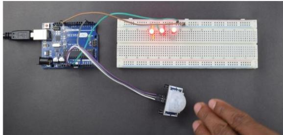
**Fig.9** LEDs glowing when the motion is detected
